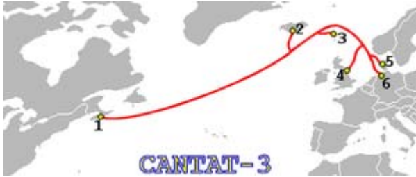
Figure 2. The Cantat 3 cable
